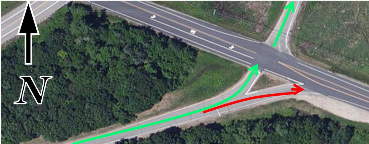
Ramp and slip ramp entering NH 155A from US 4 in Durham, and ramp entering US 4 from NH 155A. The slip ramp (marked in red) diverges from the primary off-ramp, and can only access the eastbound lane of NH 155A. The primary off-ramp (marked in green) can access either direction. Since the on-ramp can be accessed by traffic from either direction on NH 155A, it is classified as a primary ramp, not a slip ramp.
