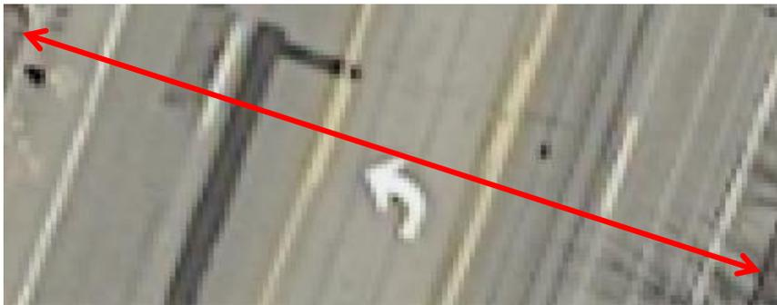
Roadway width, measured from edge of pavement to edge of pavement, including the maintained and surfaced shoulders on each side. Notice the shared-left-turn lane **is** included in the roadway width.
