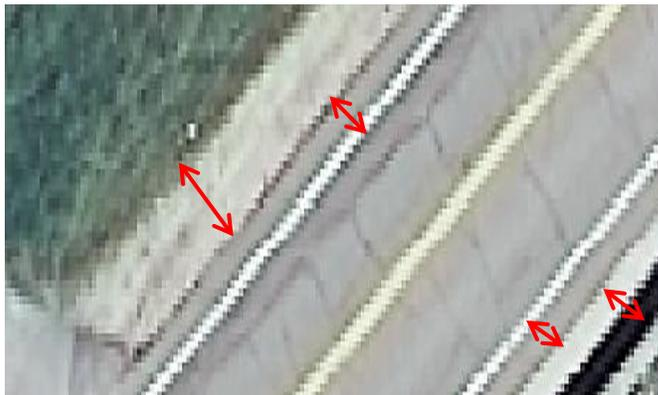
On this roadway, one can clearly see the two foot paved shoulder (which is homogeneous with the roadway surface) and the clear boarder with the gravel shoulder, which extends four feet to the left and two feet to the right. This pattern creates what is known as the combination shoulder or ‘Combo’, the predominant shoulder type in the state.
