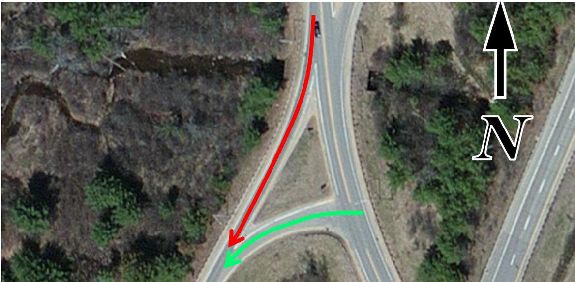
Ramp and slip ramp entering I-93 southbound from NH 132 in Northfield (Exit 19). The slip ramp (marked in red) can only be accessed while traveling south on NH 132; the primary ramp (marked in green) can be accessed from either direction. The slip ramp terminates when it meets the primary ramp. Note the island created between the primary ramp, the slip ramp, and the diverging route (NH 132).
