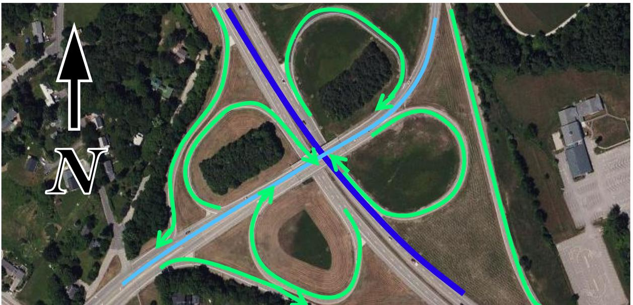
Interchange between NH 16 (shown in dark blue) and NH 9 (shown in light blue) in Dover. Each ramp (shown in green) is not a slip ramp. Despite single directions of access and egress, none of the ramps divide, and are therefore classified as primary ramps
